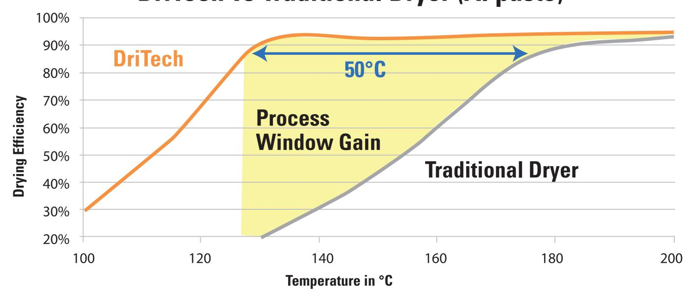
→ Dritech opens drying process window by 50°C
